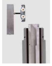
The trolley core is made from zamak and wheels from delrin, a highly resistant-to-wear material, with shielded ball bearings. Anodized aluminium fixing brackets and slide with front adjustment system. Easy access to the lateral adjustment screw allows for adjustment ease and eliminates any light infiltration above the door. Self-locking adjustment screws and adjustable nylon brake. Adjustable inferior guide. Trolley & roller tested in compliance with EN 1527 for 100.000 cycles.
